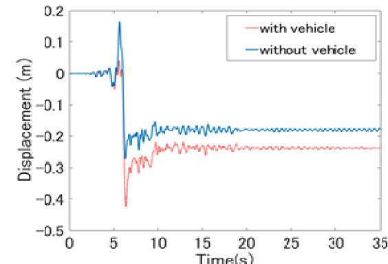
Longitudinal displacement of pier top
