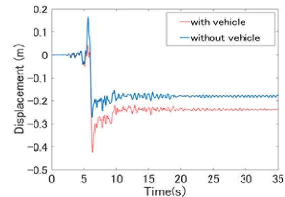
Longitudinal displacement of pier top
